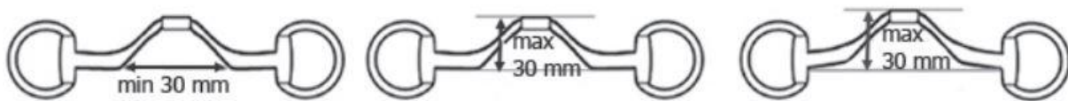
Figure 121.2: Measurement of tongue relief for a snaffle bit. The widest part of the deviation must be where the mouthpiece contacts the tongue and must have a minimum width of 30 mm (left). The maximum height of the deviation is 30mm from the lowest part of tongue side to the highest part of the deviation (center and right).
